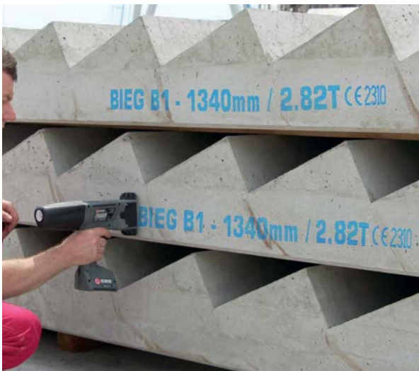
Also prints on concrete with blue pigmented ink
